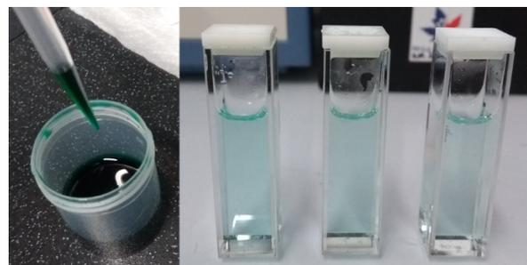
Fig. 1 An Image showing the ICG stock solution (LHS) and diluted samples in cuvettes (RHS).
