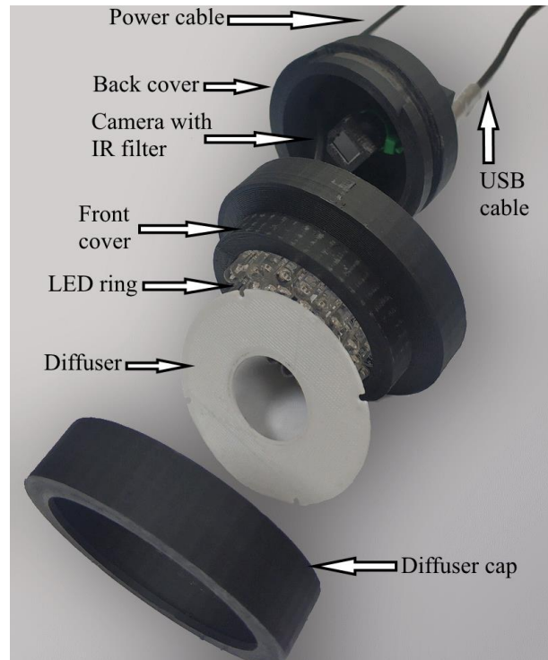
Fig. 2 Disassembled experimental stand of vein viewer.
