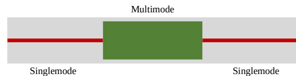
Fig. 1 SMS structure fiber optic sensor configuration.
