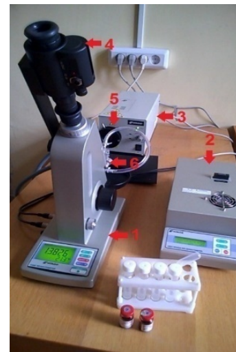
Fig. 1 General view of the experimental setup: 1 – multi-wavelength Abbe refractometer; 2 – power supply; 3 – light source; 4 – special head for measurements in the near IR range; 5 – interference filter; 6 – sample.
