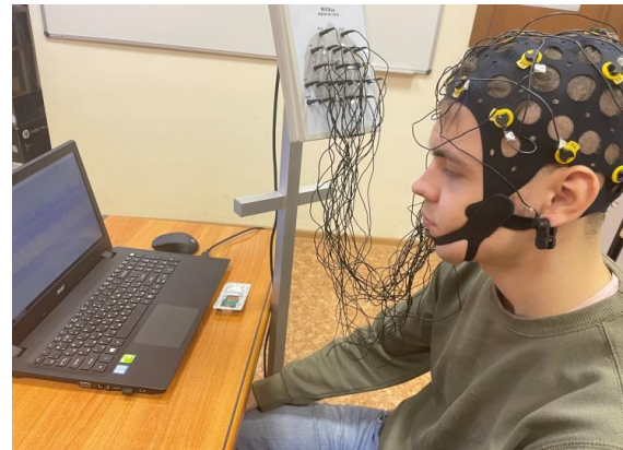
Fig. 2 Example of experimental EEG signal extraction using dry gel from MKS.
