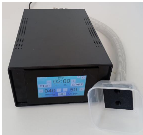
Fig. 6 Closed-loop ozone-generating system.
