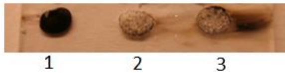
Fig. 1 (1) Absorbing coating on silica plate. Dried ( \sim 300 K) drop; (2) dried, heated at 100 \text{ W/cm}^2 ( T \sim 1000 K) and annealed at 400 \text{ W/cm}^2 ( T \sim 2000 K); (3) dried at room temperature and annealed at 600 \text{ W/cm}^2 ( T \sim 2000 K).
